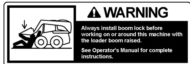
WARNING, Always Install boom Lock
